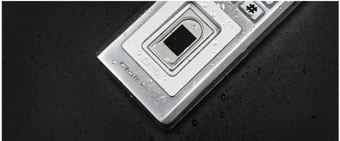
OUR PRODUCT HAS THE HIGHEST CLASS OF RAIN AND DUST RESISTANCE, IP68. IT IS RESISTANT TO EXTERNAL FACTORS SUCH AS DUST AND MOISTURE. KEEPING IN MIND THAT DUST AND MOISTURE ARE A THREAT TO ELECTRONICS, AND COMBINATION LOCKS ARE OFTEN DESIGNED FOR OUTDOOR INSTALLATION, IT IS WORTH PAYING SPECIAL ATTENTION TO THIS PARAMETER.
